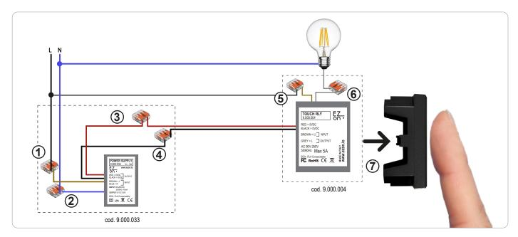
**Ezon.io Touch Relay** code 9.000.004 requires a 5vdc power supply to function (the use of the ezon.io power supply 9.000.033 is recommended).
