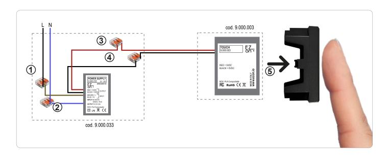
Ezon.io Touch code 9.000.003 requires a 5VDC power supply to function (we recommend using ezon.io power supply 9.000.033).
