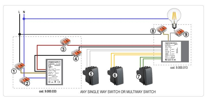
**Ezon.io Switch Relay** cod. 9.000.013 requires a 5VDC power supply to function (we recommend using ezon.io power supply 9.000.033). Connect the phase and neutral of the power supply (brown and blue cables) to the phase (black or brown) and neutral (generally blue) of your system, thanks to the quick connectors supplied with the product 9.000.033. (points 1 and 2)
