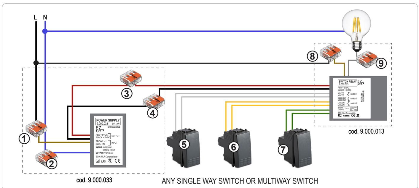
**Ezon.io Switch Relay** cod. 9.000.013 requires a 5VDC power supply to function (we recommend using ezon.io power supply 9.000.033). Connect the phase and neutral of the power supply (brown and blue cables) to the phase (black or brown) and neutral (generally blue) of your system, thanks to the quick connectors supplied with the product 9.000.033. (points 1 and 2)
