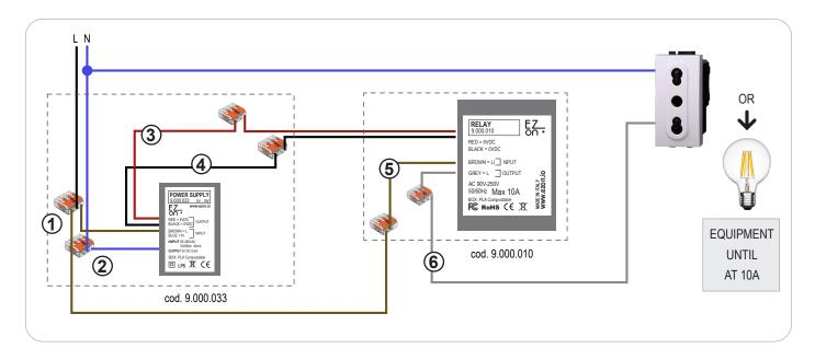
Ezon.io Relay code 9.00 0.010 requires a 5vdc power supply to function (the use of the ezon.io power supply 9.000.033 is recommended).
