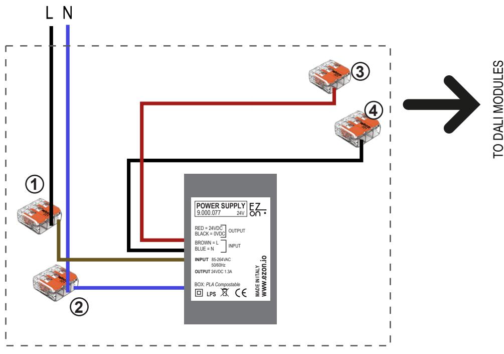
Ezon.io Power Supply 24V cod. 9.000.077 is a 24vdc power supply
