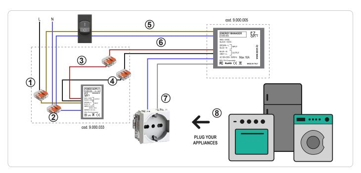
**Ezon.io Energy manager** code 9.000.005 requires a 5vdc power supply to function (the use of the ezon.io power supply 9.000.033 is recommended).
