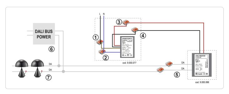
**Ezon.io Dali Bus Power** code 9.000.076 requires a 24VDC power supply to function (we recommend using ezon.io power supply 24V cod. 9.000.077).
