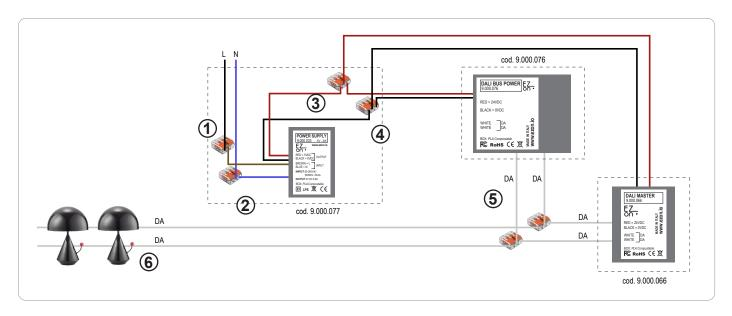
Ezon.io Dali Master code 9.000.066 requires a 24vdc power supply to function (the use of ezon.io power supply 24V cod. 9.000.077 is recommended) and a power supply for IEC62386 bus (the use of ezon.io Dali Bus Power 9.000.076 is recommended) .
