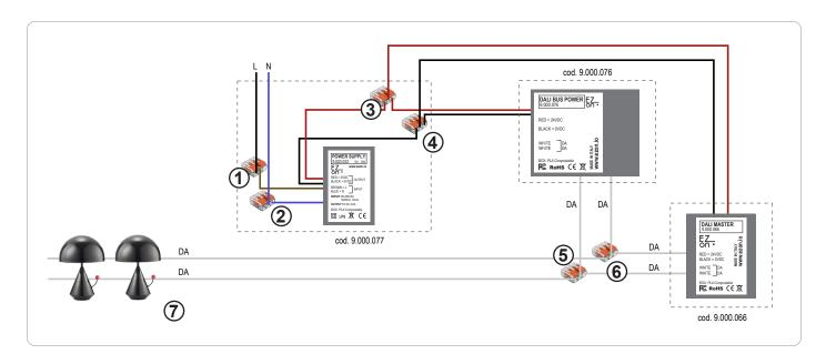
ezon.io Dali Bus Power is a power supply for Dali Bus and can be used only if in possession of a Dali Master (code 9.000.066).
