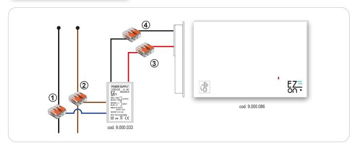
**Ezon.io T&H Sensor** [cod. 9.000.086] can determine the temperature and humidity level present in an environment. It is designed to be inserted inside a 503 cassette.
