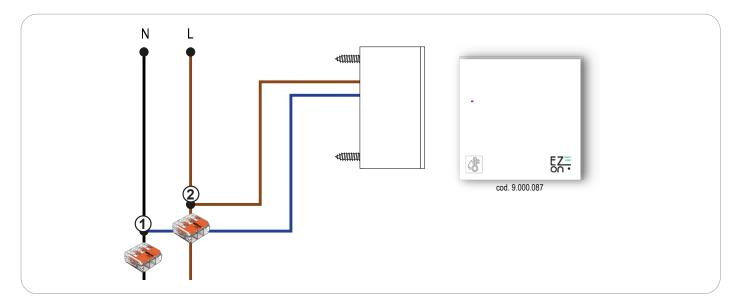
**ezon.io T&H Sensor Ezon.io** [cod. 9.000.087] can determine the temperature and humidity level present in an environment.
