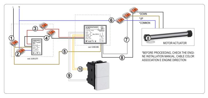
Ezon.io Motor Actuator code 9.000.028 requires a 5VDC power supply to function (we recommend using ezon.io power supply 9.000.033).
